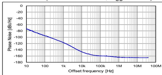
Phase Jitter (12 kHz to 20 MHz): 38 fs Typ.
