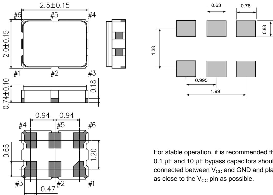
For stable operation, it is recommended that 0.1  $\mu$ F and 10  $\mu$ F bypass capacitors should be connected between  $V_{CC}$  and GND and placed as close to the  $V_{CC}$  pin as possible.
